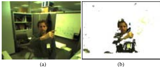
Figure 1: The original image and the same image after the disparity-based background subtraction.
